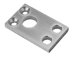
The FN Plate (Part # S9003) is made of 316 stainless steel and fastened to the end of a HD Series Type FN interlock to allow alternative mounting scenarios. The thickness of the FN Plate is 1/4". To order this plate with your HD Series Type FN interlock, put the letter "P" in the appropriate column of the interlock part number - reference the HD Series Ordering Guide. The plate (when ordered) will be bolted to your Type FN interlock.
