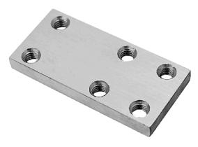
The Long D Plate (Part # S9002) is made of 316 stainless steel and fastened to the back of a multi-cylinder HD Series Type D interlock to allow front mounting (see HD Series Data Sheet 1.4). The thickness of the Long D Plate is 3/8". To order this plate with your multi-cylinder HD Series Type D interlock, put the letter "P" in column fourteen of the interlock part number - reference the HD Series Ordering Guide.
